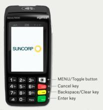
The Move 5000 has an interactive touch screen. To select a menu option simply, touch the required option on screen.
