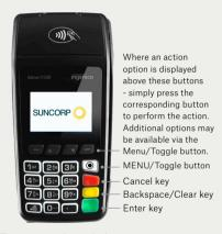
To navigate through the menu screens use the up and down arrows to highlight the required menu option and then press Enter to make your selection.
